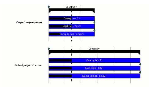
In hindsight, though fifty percent of the earth had been moved the project was actually only twenty-five percent complete in terms of the time the task would require. Earth-fill had to be moved along a narrow causeway that was being continuously extended, and dumpers could not pass each other on the narrow causeway. The further it extended the longer it took to clear the causeway for the next load.
