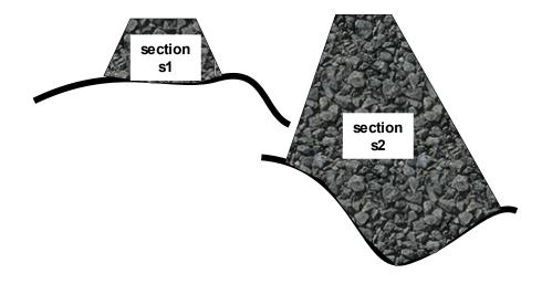
$\textit{TimeNormalizedMeasure} = \frac{\textit{SectionalArea} \times \textit{CausewayExtension} \times \textit{TimePeriod}}{\textit{VolumeDumped}}$
